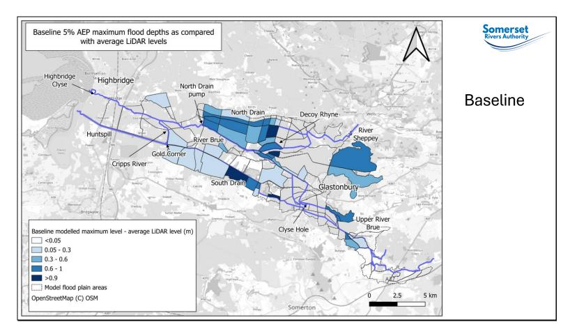
There are a lot of results that could be presented, but to simplify matters just the 5% (or 1 in 20) annual probability event is shown. The mapping just shows the average depth of flooding across different moor areas. That does not mean there isn't flooding in other areas, but it allows for an easy way to compare options.
