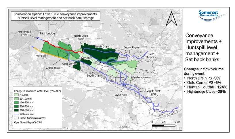
Conveyance + Huntspill + set back banks. The set back banks could be done at various locations along the Brue. This provides extra storage and also allow for the banks to be a lower height. Indicative of any option that increases storage along the Brue. Could be achieved in a variety of means. Doesn't provide a large additional benefit in this sort of event as the storage is used up early in the event, but still beneficial. Potential significant other benefits.
