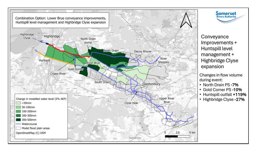
Conveyance + Huntspill + Highbridge. Widening Highbridge Clyse reduces a major constriction and provides additional conveyance at low tides. A much more challenging project to implement.
