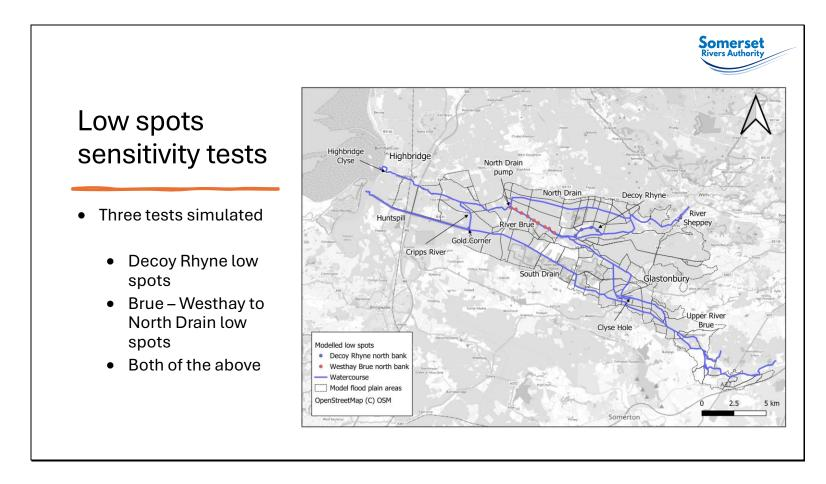
Assessed approximate frequency of low spots based on Brue walkover survey around Westhay and applied this throughout with localised short sections of bank lowered in the model.
