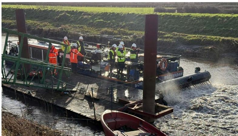
The Borr then uses powerful jets of water to agitate and disperse the material placed in its path, so they get washed out on the outgoing tide. The water injection bar is shown in the raised position.
